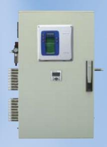
The multi-point system uses the same sampling arrangement as the single point system, but can monitor up to 16 separate sample lines on a sequential basis. The multi-point system provides a cost effective and low maintenance solution for monitoring gas hazards in buildings, pumping stations, storage areas etc.
